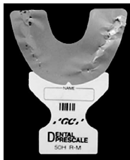
Fig. 2. Fuji film Prescale after pressure measurement
